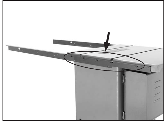
Figure 11. Rear rail installed.
